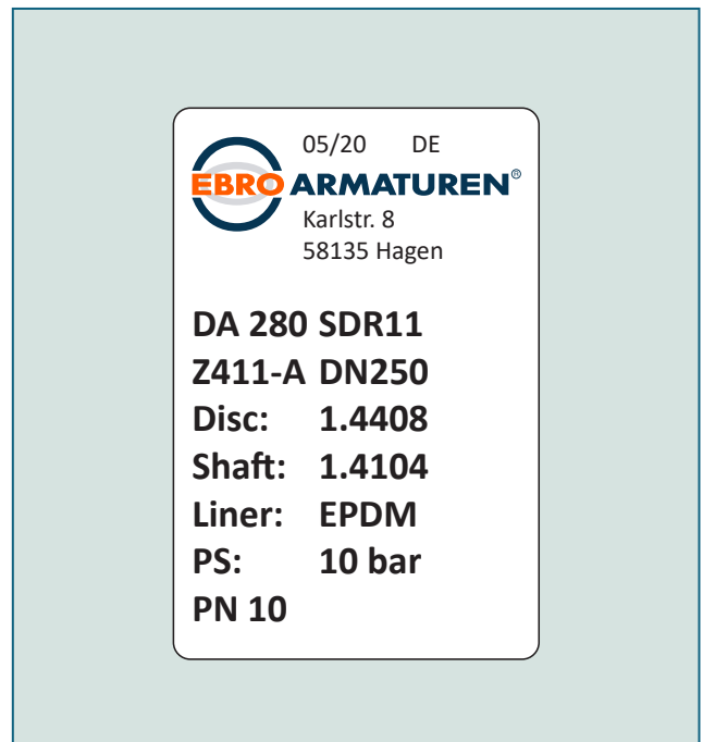
Type plate for clear identification of the Z411-A.
